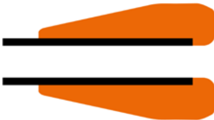
Diagram of external PTFE bush fitted to pole tip
